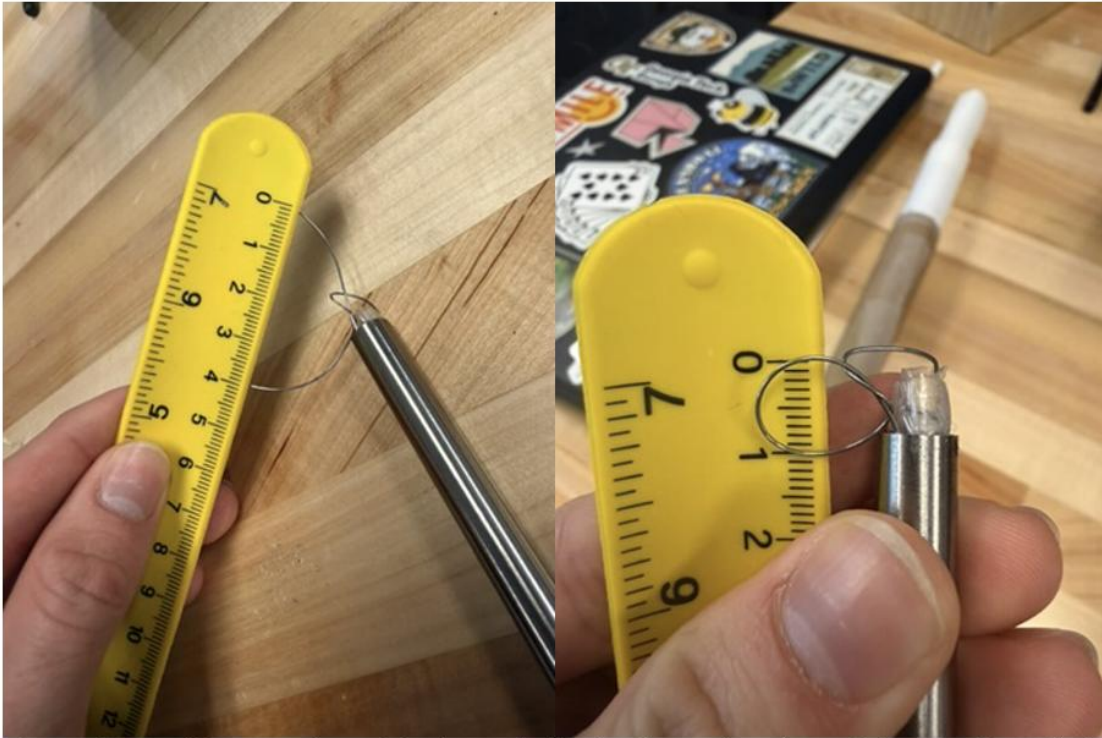
Figure 15. Rapid prototyping of the dynamically sized resection electrode loop testing. The left shows the largest diameter being measured to be 4cm. The right shows the smallest loop diameter being measured to be about 1cm.
