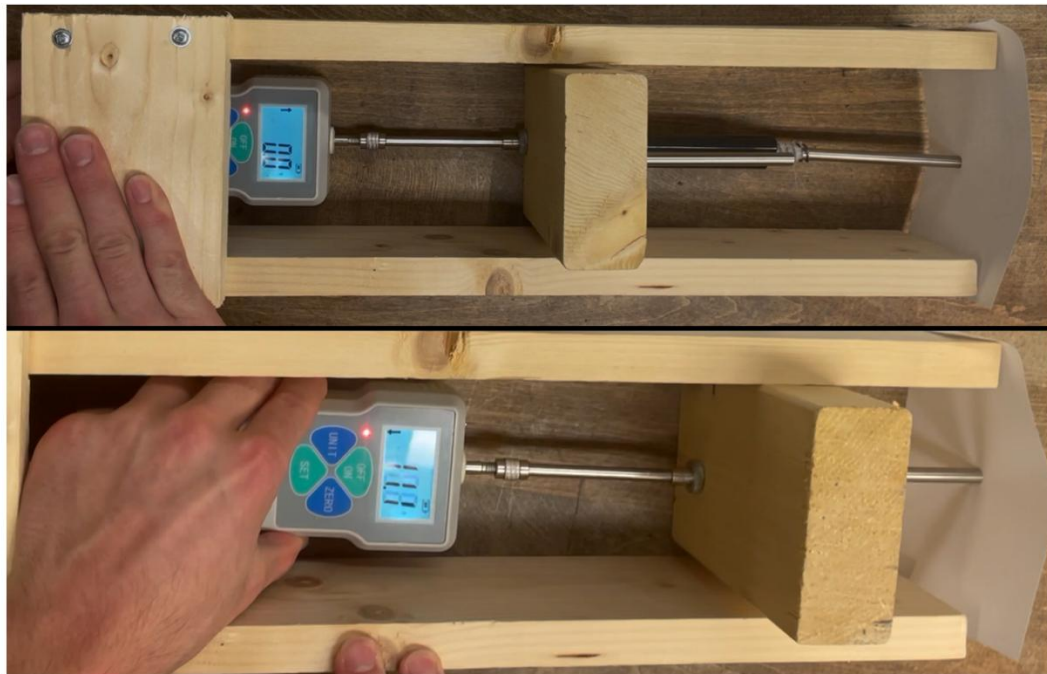
Figure 7. Rapid prototyping spring sheath perforation force testing. The top features the spring sheath prior to applying a force to a sheet of paper. The bottom shows the control sheath applying a force to a piece of paper. The force gauge readings were recorded until the paper samples were perforated, and the maximum forces were identified and compared. The mean and standard deviation of the perforation forces for the spring sheath and control sheath were 17.93 \pm 1.07 N and 21.73 \pm 0.71 N, respectively.
