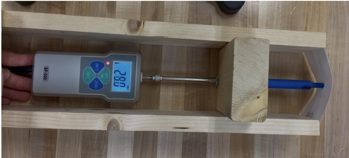
Figure 24. Generation 1 spring sheath perforation force testing. The same setup was used as for the low-fidelity spring sheath model. The mean and standard deviation of the perforation forces for the spring sheath and control sheath were 23.68 \pm 8.18 N and 19.00 \pm 2.61 N, respectively.
