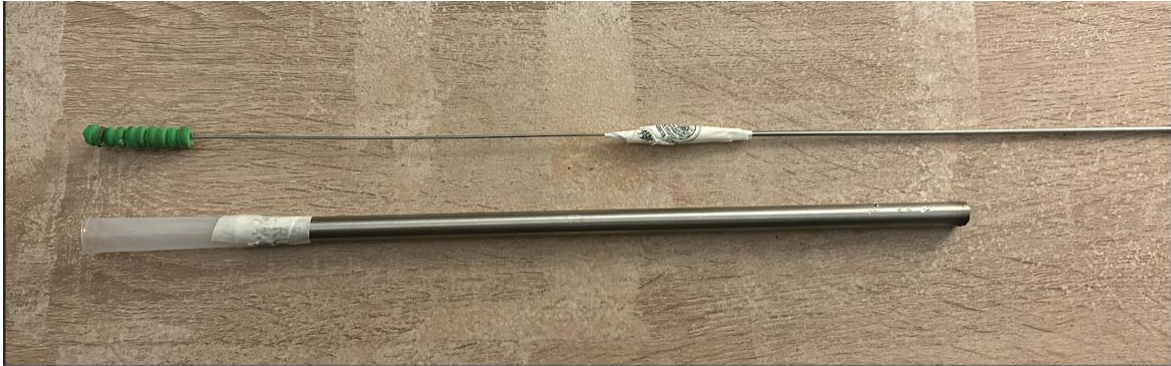
Figure 10. Rapid prototype of force limiting compliant tip containing a distal tip composed of a graded-stiffness material.
