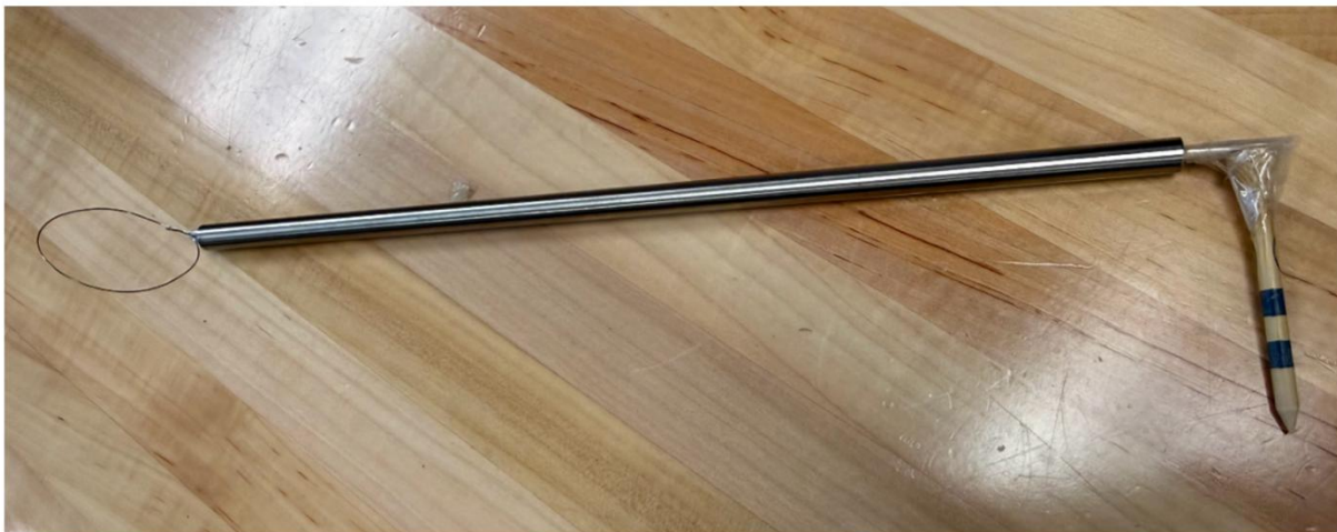
Figure 14. Rapid prototype of dynamically sized built-in resection electrode hysteroscope
